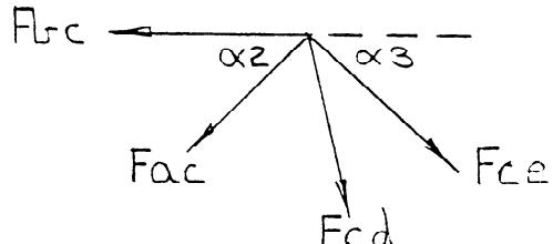
$$F_{ac} = -61.85 \text{ kN (compressive)}$$
