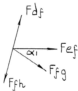
$$4.26 \times 0.986 = F_{fg} \times 0.479 + F_{fh} \times 0.986$$
